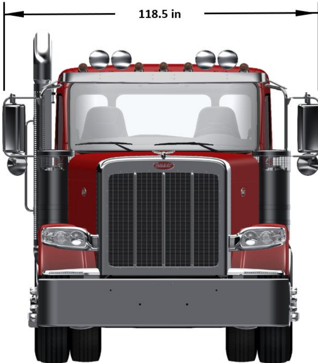
FIGURE 3-3. Model 589-131 Front View – Overall Dimensions
