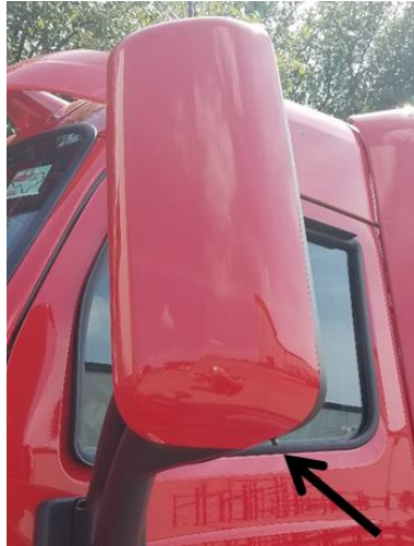
FIGURE 2-3: Aerodynamic Mirror OAT Sensor Location
